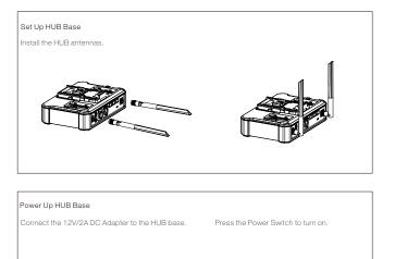
Note: The HUB Base can be powered using NP-F battery, V-Mount/G-Mount battery, or DC power supply.
