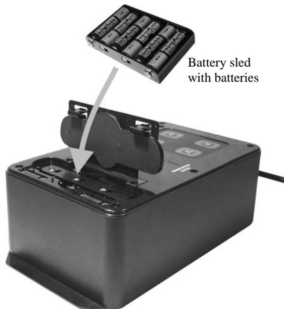
Close the battery compartment by pressing its cover down until both latches snap in place.
